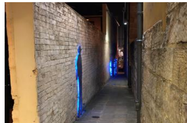
Figure 7.172 Integrated coloured linear LED to the wall featured of Suez Canal creates intrigue in the narrow passageway
