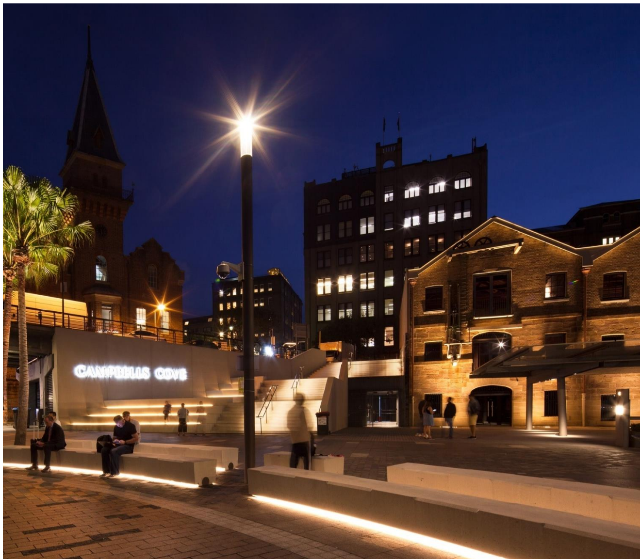
Figure 5.10 Lighting at Campbell's Cove showcasing a mix of lighting types including in-ground and integrated lighting, pole lighting and backlit signage, Brett Boardman
