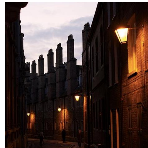
Figure 7.149 Accent lighting highlighting architectural features and grazing the surface of the brick and stone façade, Thomas Heyl
